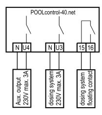
An auxiliary item of equipment running at 230V (e.g. underwater lighting) can be connected to terminal U4 and can then be timed to switch on and off by a dedicated timer in the control unit. Since this is a configurable output, it can also be used for controlling a floculation pump.
