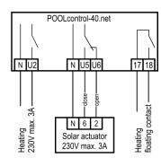
The pool heating can be connected to the terminal U2. This output supplies 230V and is rated for a maximum load of 3A.
