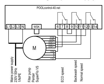
A SuperFlo VS pump can be controlled by the PC-40.NET unit.
