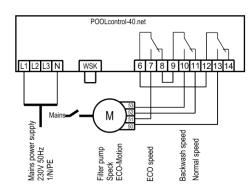
A Speck ECO-Motion pump can be connected directly to the PC-40.NET unit. Connect the speed controller to terminals 6-13.
