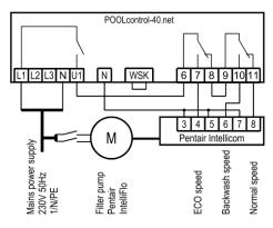
An IntelliFlo pump can be controlled by the PC-40.NET using the Pentair Intellicom controller.
