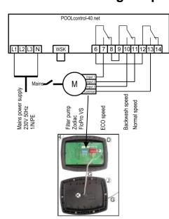
A Zodiac FloPro VS pump can be connected directly to the PC-40.NET unit. Connect the speed controller to terminals 6-13.
