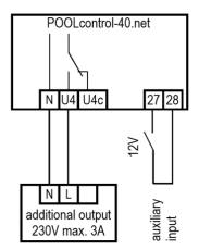
An additional load, such as lighting, can be connected to terminals U4 and N. This output provides 230V and can be used up to max. 3A burdened.
