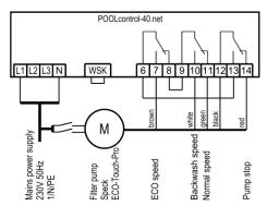
A Speck ECO-Touch-Pro pump can be connected directly to the PC-40.NET unit. Connect the speed controller to terminals 6-14.
