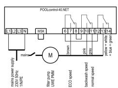
A UWE PMM pump can be controlled by the PC-40.NET.
