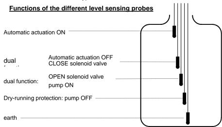
In normal mode, the water level fluctuates between the "CLOSE solenoid valve" and "OPEN solenoid valve" probes.
