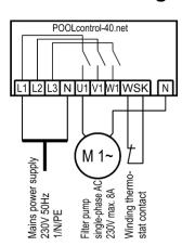
The factory-inserted link between the two WSK terminals must be removed when connecting a pump fitted with a thermal winding protection switch (winding thermostat). If the pump does not have a winding protection switch, the link must remain screwed in place. These terminals are live and carry a mains voltage!
