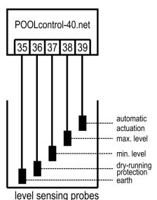
electrode probes must be used as the level sensors.
