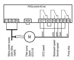
A Speck ECO-VS pump can be connected directly to the PC-40.NET unit. Connect the speed controller to terminals 6-14.
