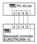
A 4-wire connection is required for connecting the EUROTRONIK-10. The wires must not be swapped over, i.e. they must be connected to the same terminal at each end. The EUROTRONIK-10 additionally requires a separate power supply.
